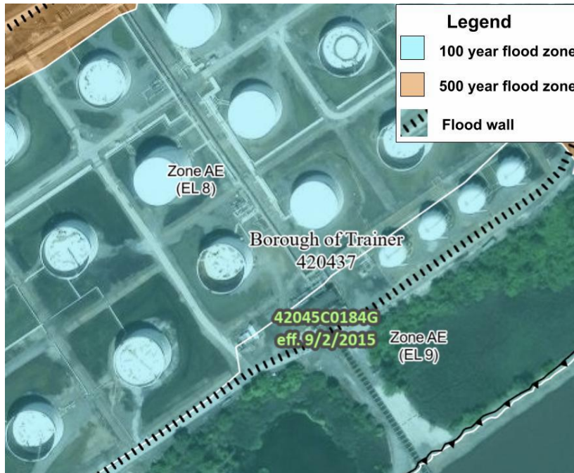
Figure 10. FEMA flood risk map of Monroe Energy Trainer Facility showing their 24 oil storage tanks behind inadequate flood walls
