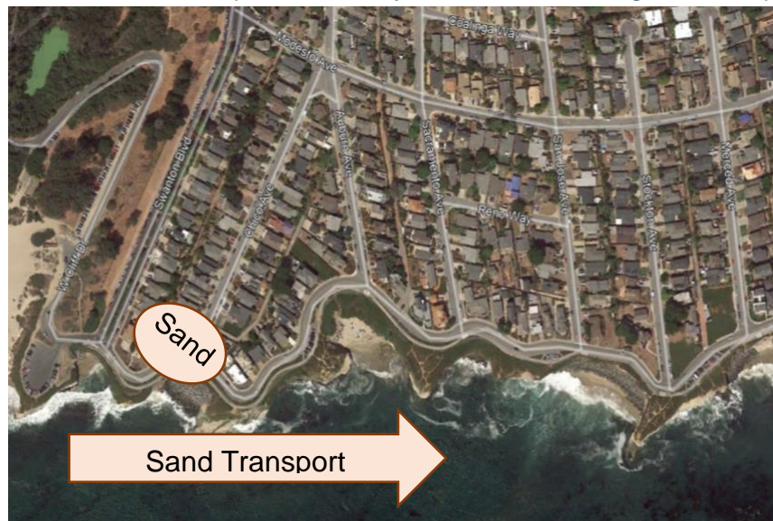
Figure 2-9. Potential sand placement at Pyramid Beach with longshore transport
