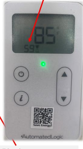
If you want to stop occupied timer, push a second time and "0" will show, which puts the time to zero minutes and the system will revert to unoccupied mode.
