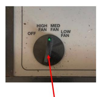
You will see this switch under the cover. Adjust to the speed desired, remember not to shut off.
