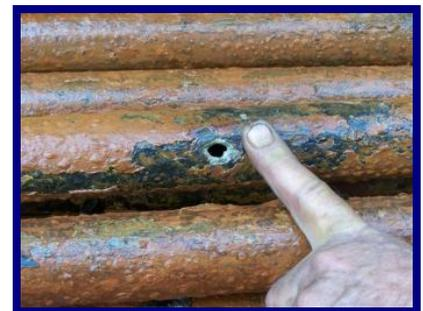
*Hole in corroded well pipe.*
